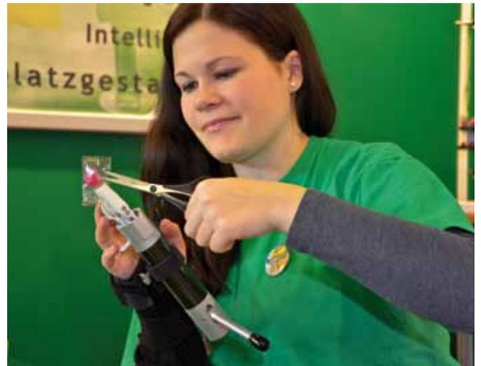
Whether the grip function is restricted uni- or bilateral, the use of the Gripability b.hand is recommended, whenever the application of a compact and mobile gripping and grasping aid leads to an extension of the capacity of physical action.
